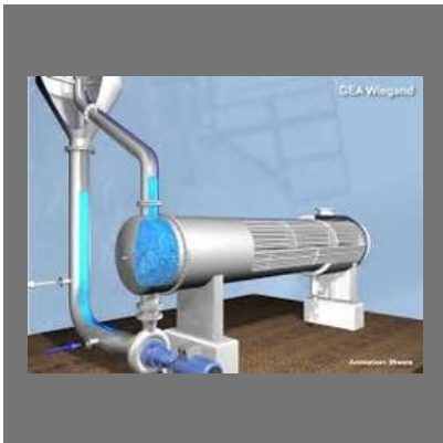
Forced Circulation Evaporation Plant
